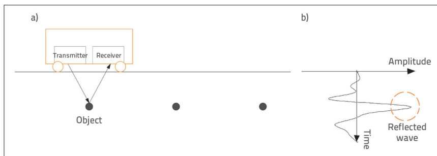
Figure 3. a) GPR system, b) A-scan
