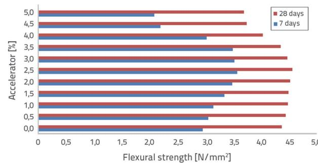
Figure 8. Variation of Flexural strength with various % of accelerator
