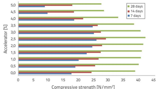
Figure 5. Variation of compressive strength with various % of accelerator
