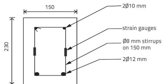
Figure 1. Cross-section of the beam
