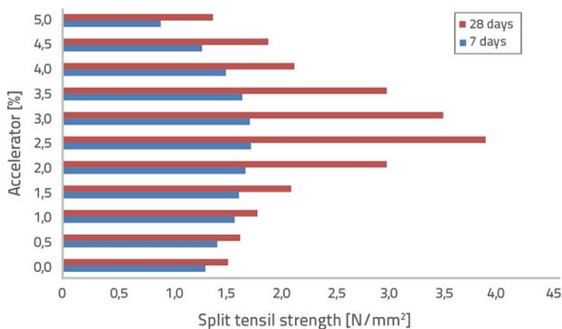
Figure 7. Variation of Split tensile strength with various % of accelerator
