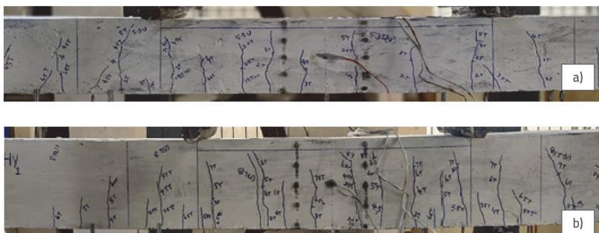
Figure 10. Crack characteristic of: a) CC beam; b) A2.5 % beam
