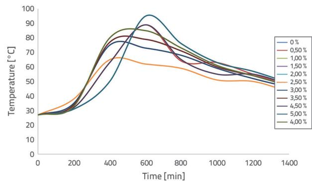
Figure 3. Heat of hydration
