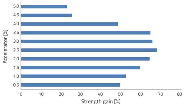
Figure 6. Strength gain of mix with various % of accelerator
