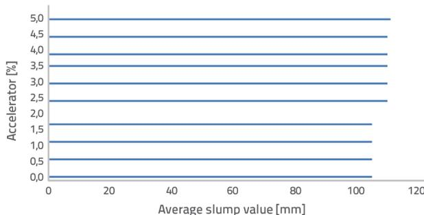
Figure 4. Variation of Slump Values with various % of accelerator
